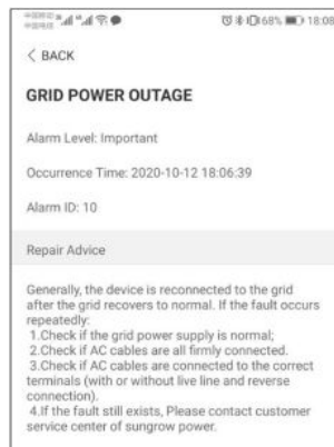
figure 7-9 Detailed Fault Alarm Information
