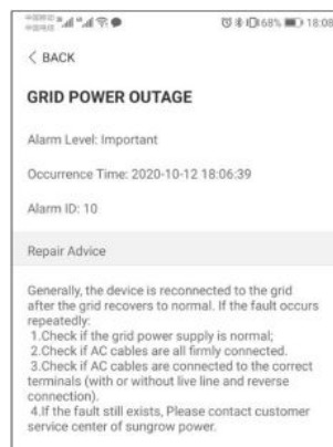
figure 7-9 Detailed Fault Alarm Information
